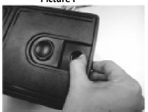
Snap front panel down into the frame and push the latch to the right to lock.
