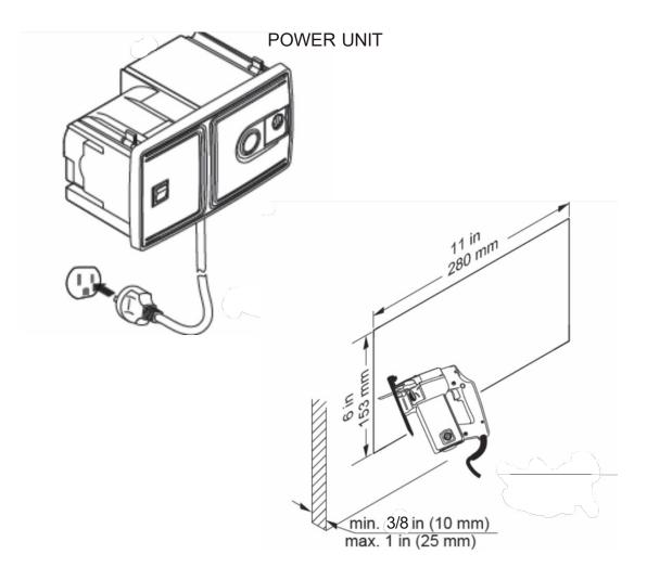
The central vacuum should be mounted so that power supply cord can be plugged directly into an electrical outlet.
