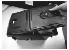
Slide front panel with left side into the vacuum frame. Watch out that the bag does not get champed between front panel and frame!
