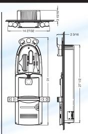
When using our optional flush mount installation kit (A-702) you can easily install it inside of a 2x4 studded wall. (basic carpentry skills required).
